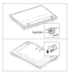
Screw length from outer surface of back cover should be under 8 mm. (Only 24/28LN66\*)
